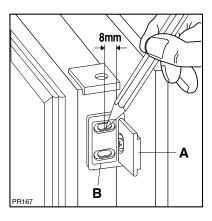
Should adjustment of the furniture door be necessary, use the clearance of slots as required.
